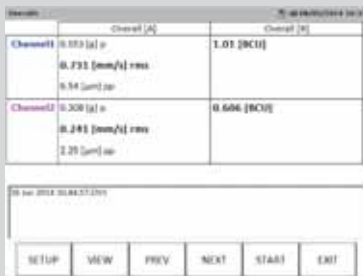
Two-channel real overall measurements (bandpass/BCU)
